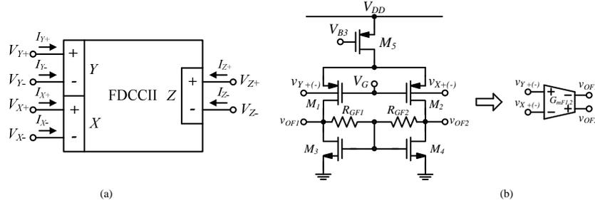
Fig. 2. (a) The Symbol of FDCCII and (b) bulk-driven feedforward transconductor.
