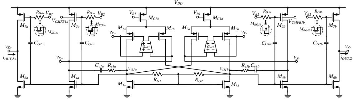
Fig. 1. Bulk-driven CMOS FDCCII with feedforward circuit.
