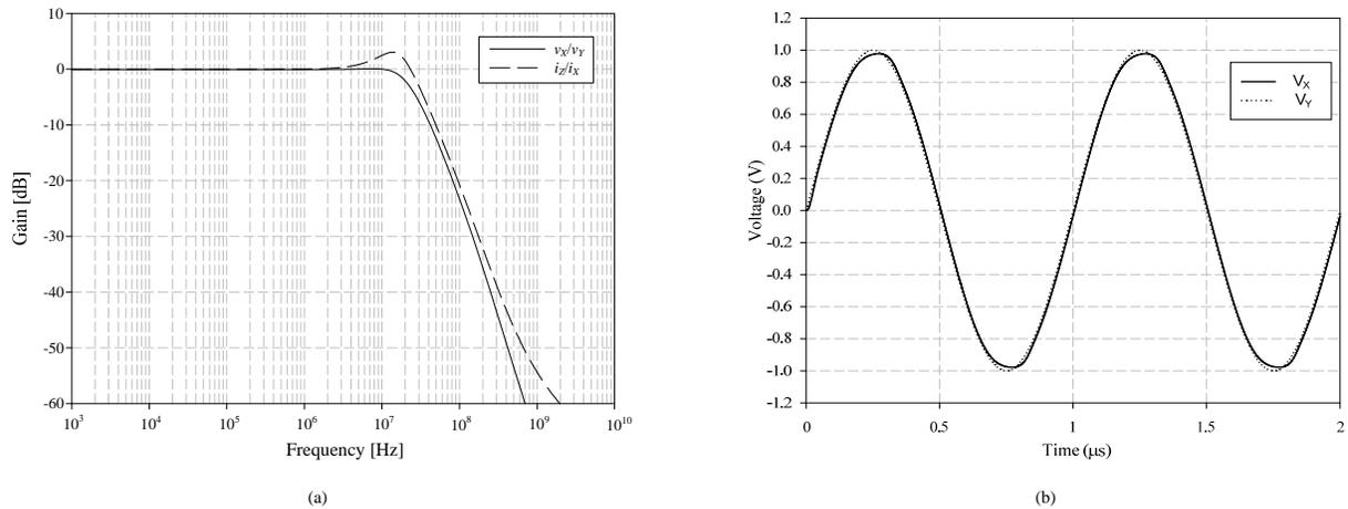
Fig. 5. (a) Frequency response of  $v_x/v_y$  and  $i_z/i_x$  and (b) Transient response (Input 2 V<sub>pp</sub>, 1 MHz).
