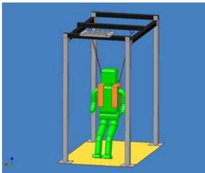
Figure 7. The model of low-cost parachute training simulation system
