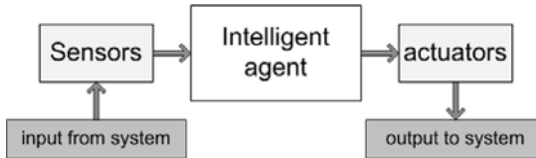
Figure 1.2 Typical artificial intelligent agent diagram that receives information through sensors and provides responses through actuators. When applied to a radio system, the agent provides the cognition to the cognitive radio.
