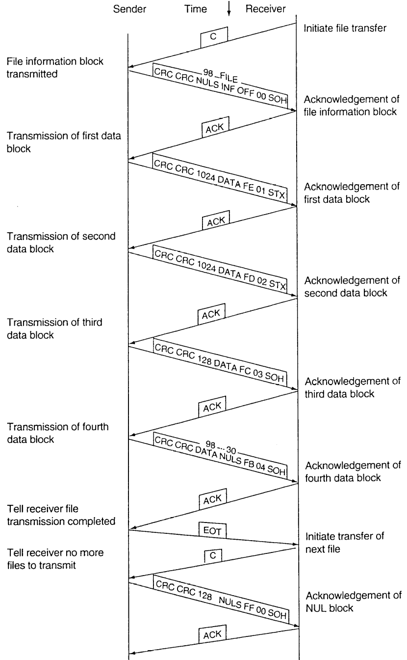
Figure 11.5 YMODEM protocol file transfer example
