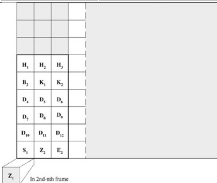
Figure 27-7: The line overhead of a SONET frame
