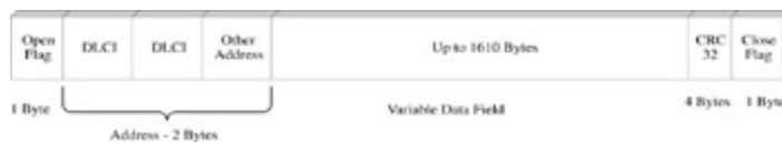
Figure 10-4: A Frame Relay frame
