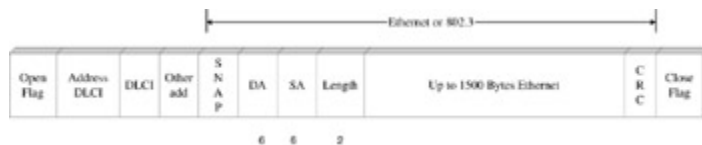
Figure 10-5: Ethernet and IEEE 802.3 frames fit into the Frame Relay frame
