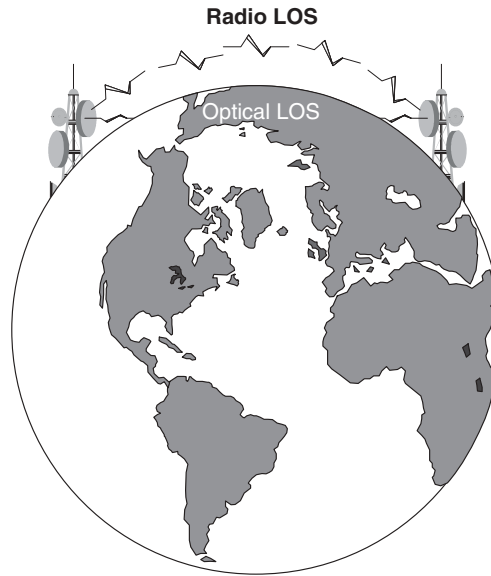
Figure 2.9 Microwave path illustrating differences between optical and radio LOS.
