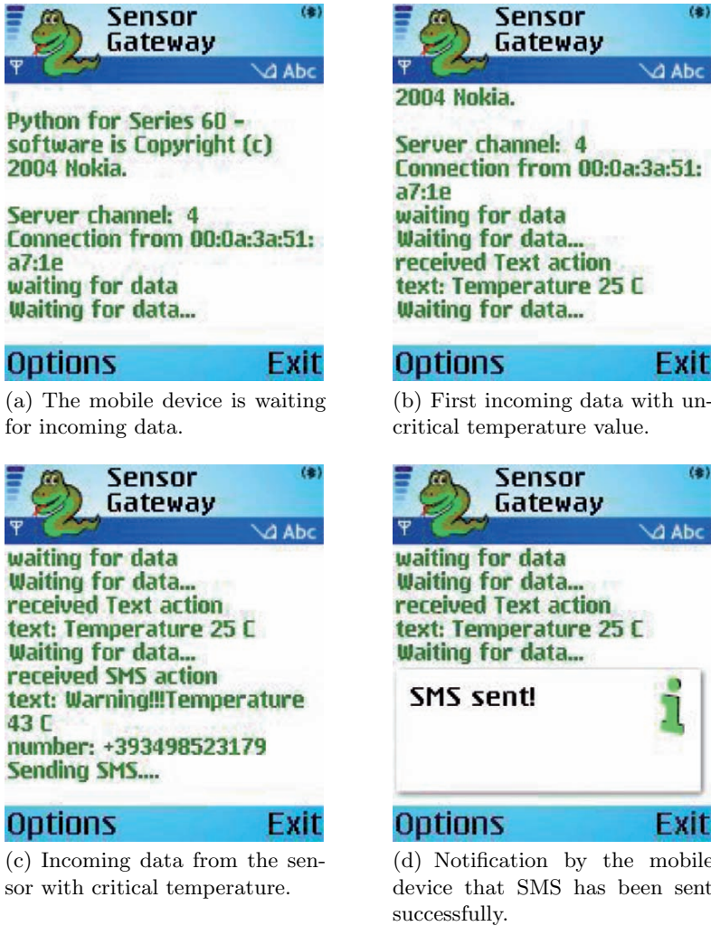
Figure 19.4. Screenshots of the sensor gateway realization
