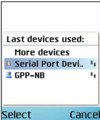
(c) Select the device to connect to. In this case the sensor is represented by the “Serial Port Device” entry in the list of Bluetooth devices found.
