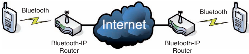
Figure 12.2. The Internet link scenario describing two mobile phones, connecting over the Internet using Bluetooth.
