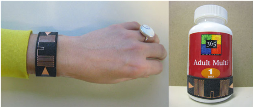
Fig. 13.2 Embodiments of the conformal RFID tag prototype in the applications of wireless health monitoring and pharmaceutical drug bottle tracking
