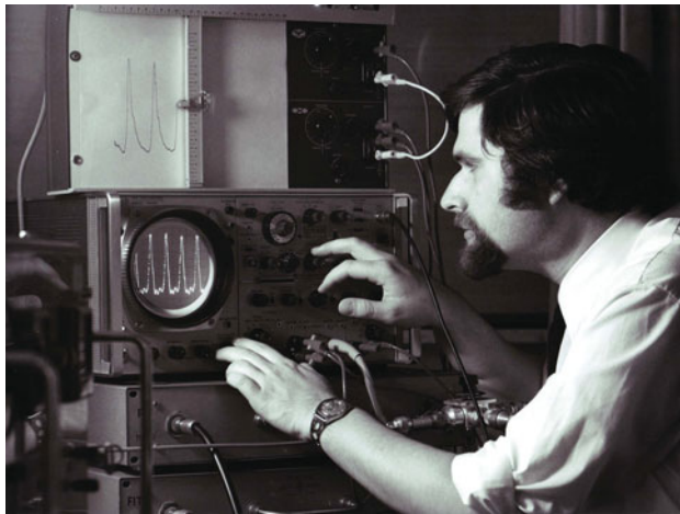
Fig. 8 At the experimental investigation of the direct modulation of a semiconductor injection laser with a bit rate of 500 Mbit/s in the year 1972
