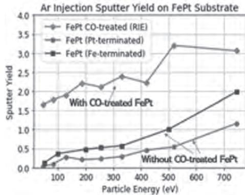
Figure 2. FePt sputter yield (with Ar ions) comparison on CO/H<sub>2</sub>-treated and non-treated surface
