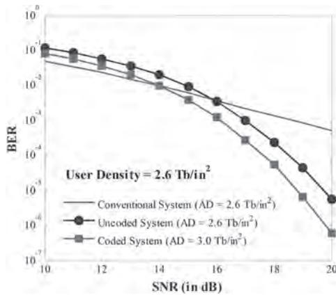
Fig. 2. Performance comparison of various systems at UD = 2.6 Tb/in<sup>2</sup>.
