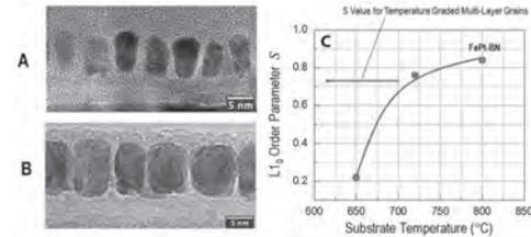
Figure 1 (A) Out of plane micrographs of FePt-BN (8 nm) (B) Out of plane micrographs of FePt-BN/FePt-SiO<sub>2</sub> (11 nm) and (C) Order parameter Vs set temperature of FePt-BN sample
