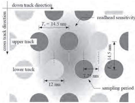
Fig. 1. Configuration of the proposed DTR systems at AD = 3.0 Tb/in<sup>2</sup> under the readhead sensitivity response that is positioned between the desired upper and lower tracks.
