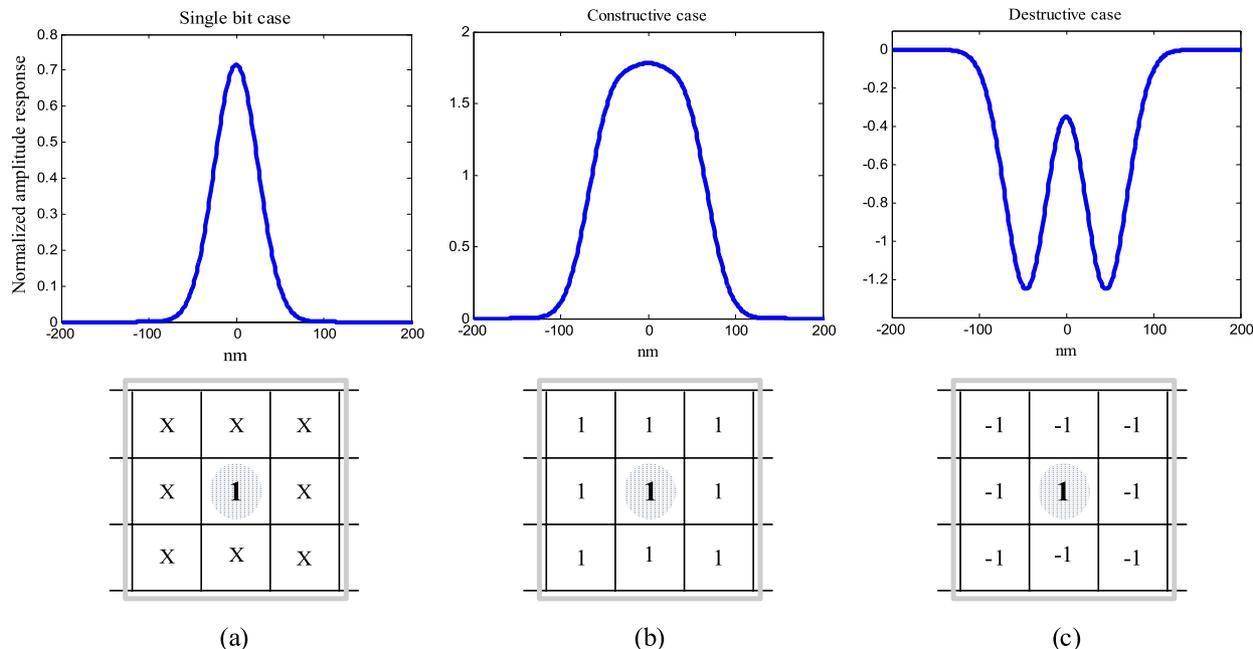
**Fig. 1** Examples of the readback signal of (a) the single bit case, where ‘X’ denotes no recorded bit, (b) the constructive interference case when the bit “1” is surrounded by all 1’s, and (c) the destructive interference case when the bit “1” is surrounded by all -1’s. All readback signals are generated based on the channel model in Fig. 2 without noise.
