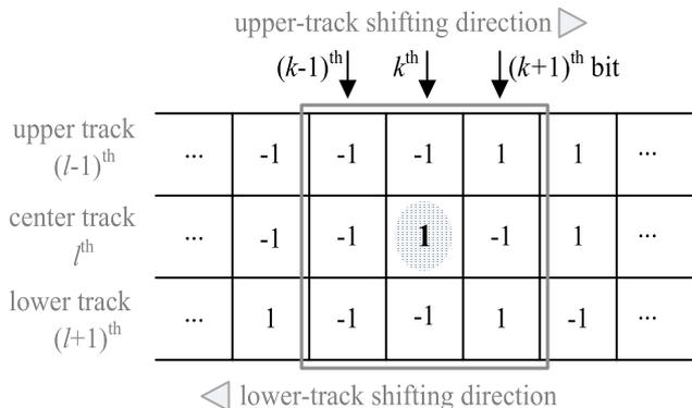
**Fig. 3** A simple RBP scheme, where the  $l$ th center track is fixed, and the ( $l-1$ )th upper track and the ( $l+1$ )th lower track are circularly shifted to the right and to the left, respectively, to create all possible 3-track data patterns.
