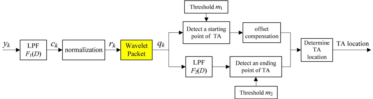
Fig. 3. The diagram of the TA detection and location block.
