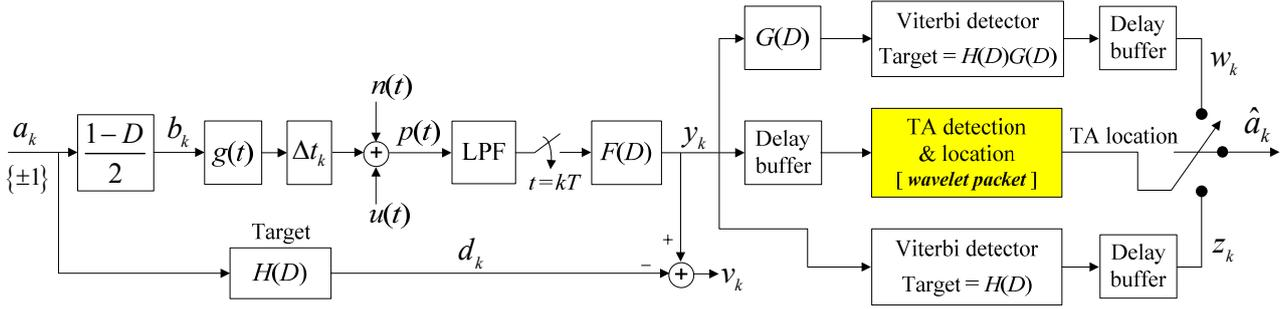
Fig. 1. Channel model with the proposed TA suppression method.
