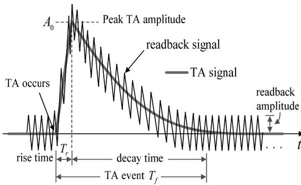
Fig. 2. The TA signal  $u(t)$  associated with the MR sensor head.
