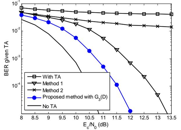
**Fig.6:** Performance comparison of different TA suppression methods in coded systems.
