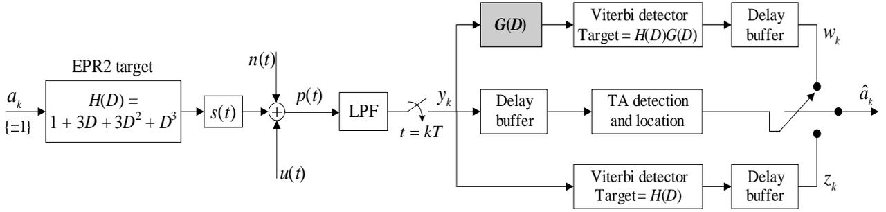
Fig. 1: A channel model with the proposed TA suppression method.
