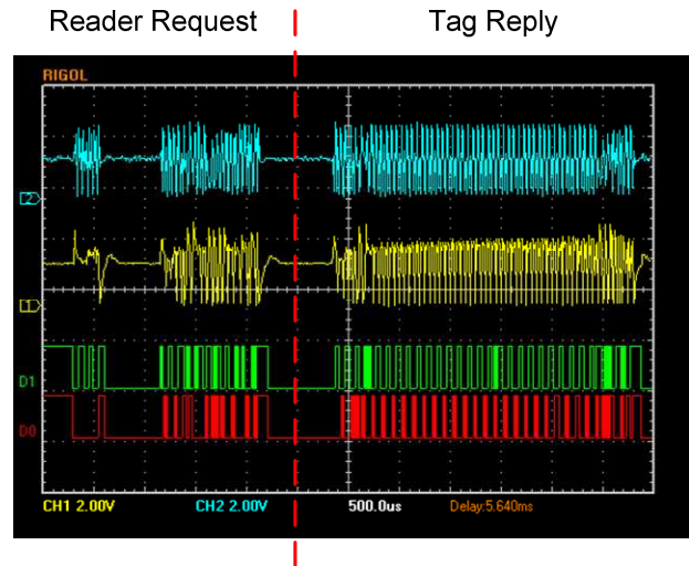
Fig.8: Analog and Digital Signals Transmit and Receive between A Reader and A Tag.
