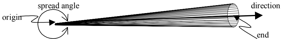
Figure 4-15 Parameters of PickCone pick shapes
