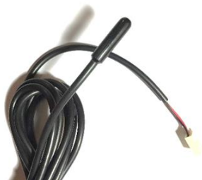
Fig. 5. DS18B20 Temperature sensor from Dallas Semiconductor.
