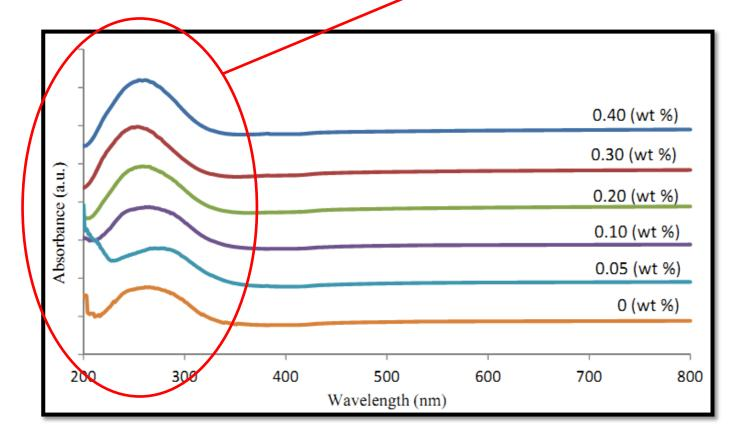
Fig. 16 The optical spectra of ZnO-doped glass
