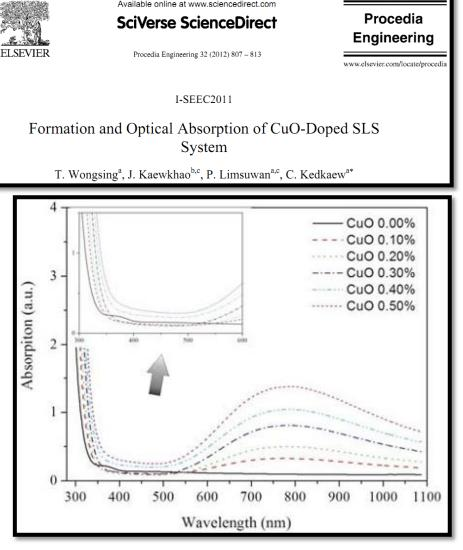
Fig. 14 The optical spectra of CuOdoped glass
