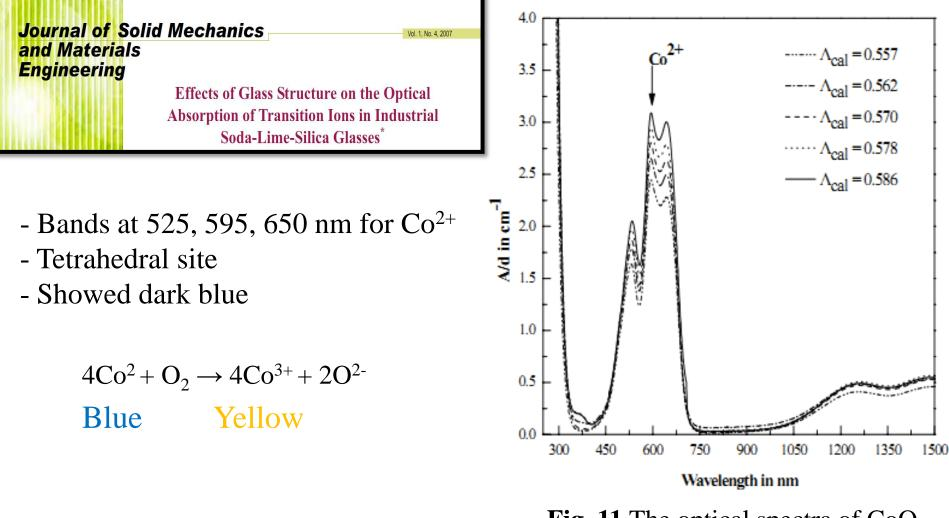
Fig. 11 The optical spectra of CoOdoped glass Advanced Materials Research Vol. 979 (2014) pp 275-279 © (2014) Trans Tech Publications, Switzerland doi:10.4028/www.scientific.net/AMR.979.275
