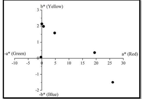
**Fig. 8** The CIE L\*a\*b\* color scale of MnO<sub>2</sub>-doped glass
