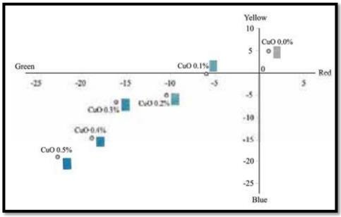
**Fig. 12** The CIE L\*a\*b\* color scale of CuOdoped glass
