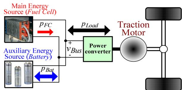
**Fig. 1:** Fuel cell hybrid power source for distributed generation system. ( $p_{Load}$ ,  $p_{FC}$  and  $p_{Bat}$  are the load, fuel cell, and battery powers and  $v_{Bus}$  is the DC bus voltage.)
