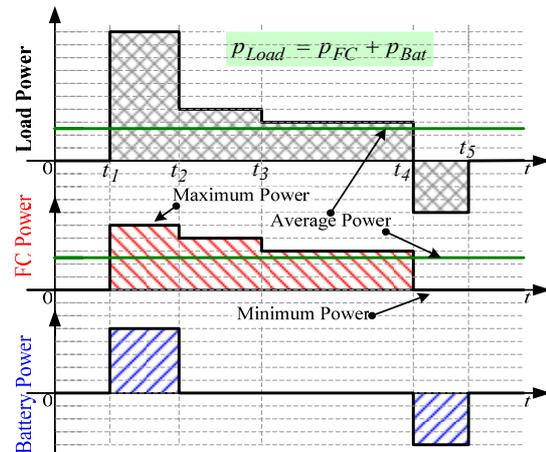
**Fig. 2:** Power profile of fuel cell hybrid source.
