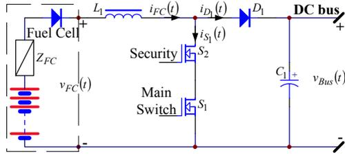
Fig. 4: FC power conditioning (FC converter) [3].
