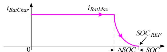
Fig. 5: Charging battery algorithm.
