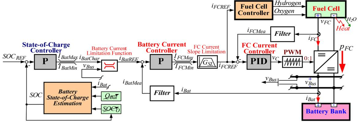
Fig. 3: Proposed control structure of fuel cell/battery hybrid power source.
