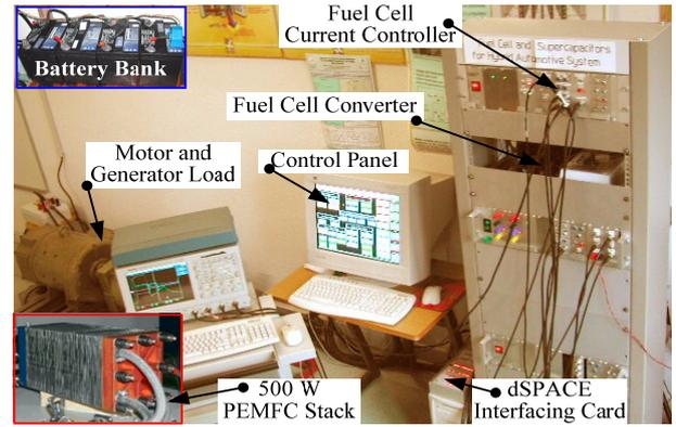
Fig. 6: Hybrid source test bench.
