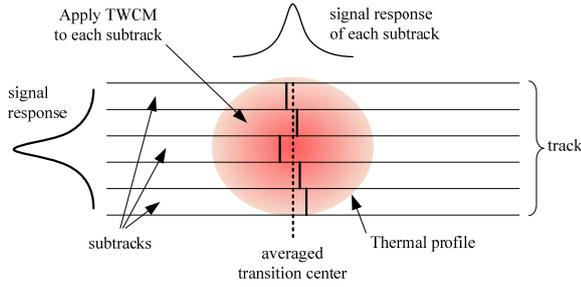
**Fig. 2.** A microtrack model with thermal profile.
