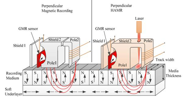
**Fig. 1.** Perpendicular magnetic recording (PMR) and perpendicular HAMR system.
